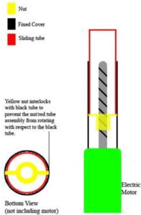
Fig actuator mechanism
