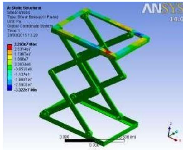
Fig No-4, Shear stress analysis
