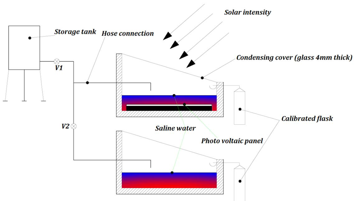
Fig. 1 Schematic diagram of hybrid and conventional solar still
