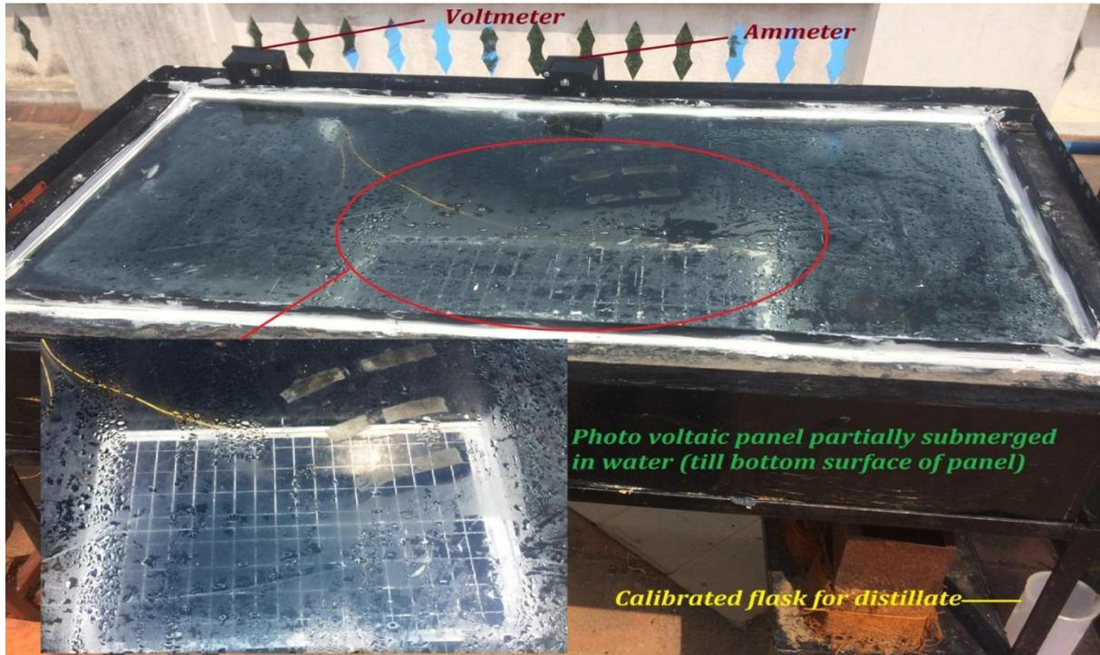
Fig. 2 Experimental photograph of hybrid solar still with water
