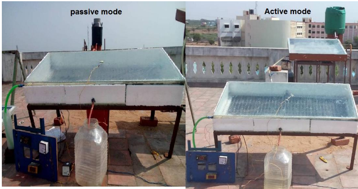
Fig. 2 Experimental set-up of inclined Solar panel basin solar still in passive and active mode
