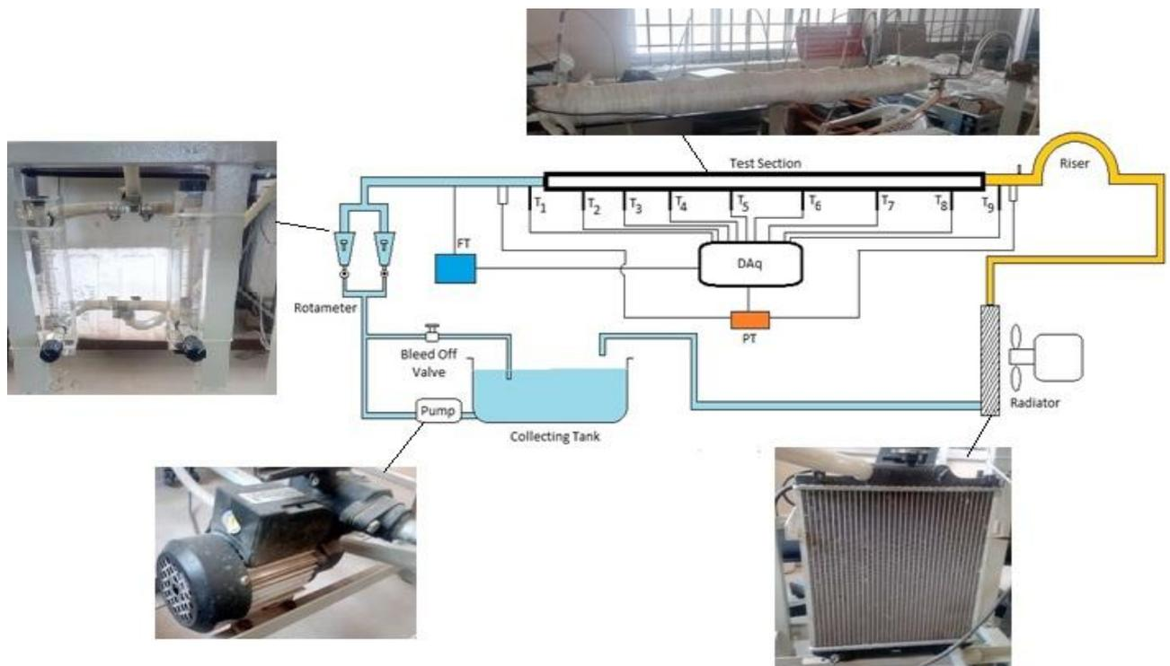
Fig. 2. Schematic diagram of heat transfer apparatus
