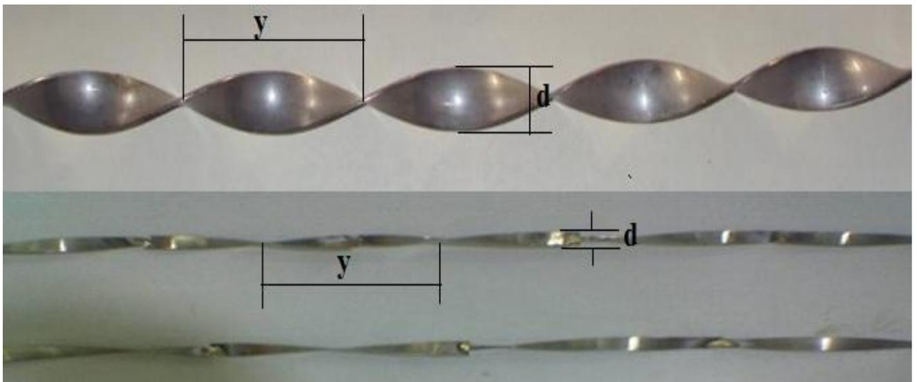
Fig. 3. Straight and Left-Right twisted tapes used in present work
