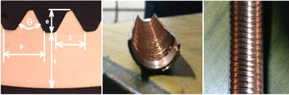
Fig. 1. Micro-fin tube used in present work
