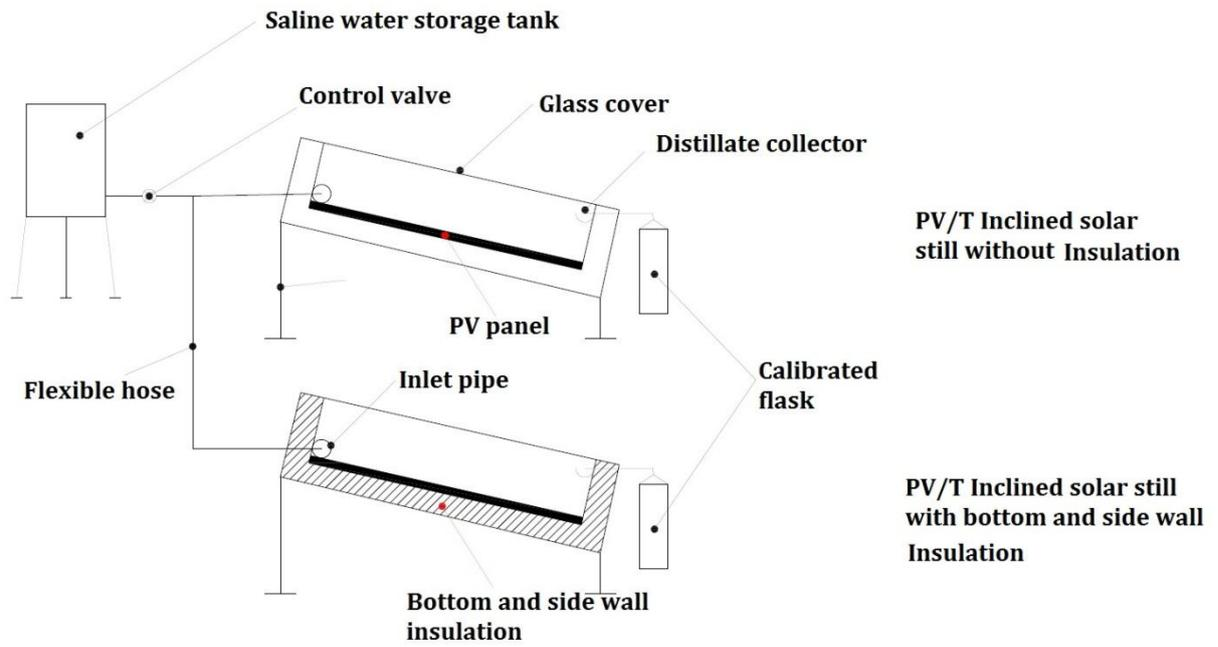
Fig. 1 Schematic diagram of modified PV/T solar still with and without insulation
