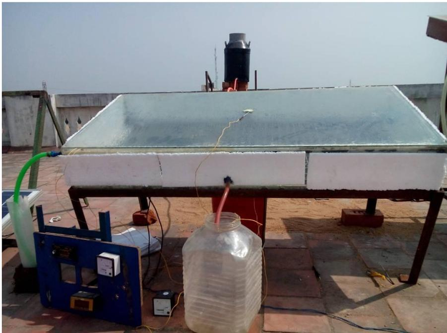
Fig. 2 Experimental set-up of inclined Solar panel basin solar still with insulation
