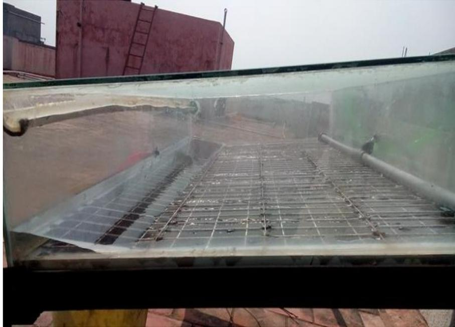
Fig. 3 Water flowing arrangements in solar panel basin solar still.
