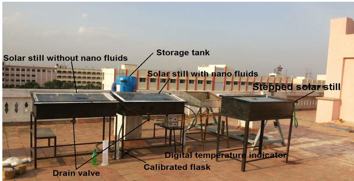
Fig. 1 Experimental photograph of different solar still arrangement
