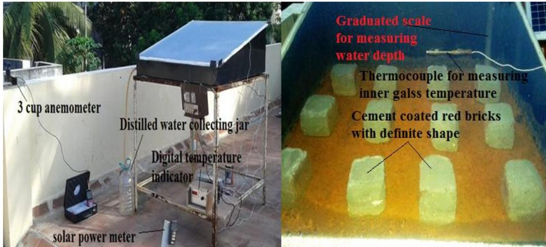
**Fig. 2** Experimental photograph of the modified solar still with instrumentations used
