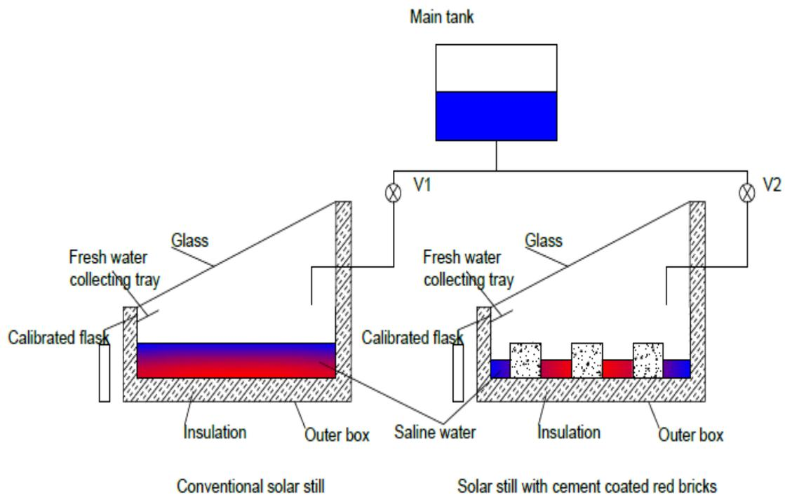
**Fig. 1** Schematic diagram of conventional and modified solar still with cement coated red bricks
